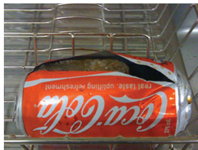
Figure 3. A Coke can that has split after freezing.
